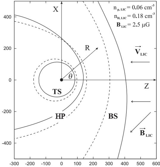
**Fig. 1.** The structure of the heliospheric interface. TS is the termination shock, HP is the heliopause and BS is the bow shock. Solid curves correspond to the model, when the interstellar magnetic field is taken into account, dashed curves correspond the model with vanishing magnetic field.
