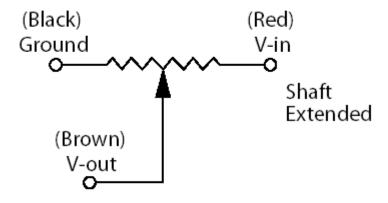
Connect to High Impedance Circuit
