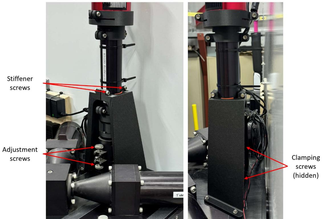
Figure 6: Slit viewer focus adjustment elements. The clamping screws should be accessible with a ball end hex wrench behind the twisted stiffener.
