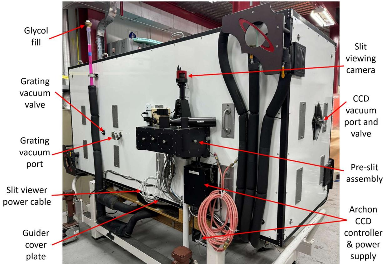
Figure 2: The side of PFS that faces the telescope.
