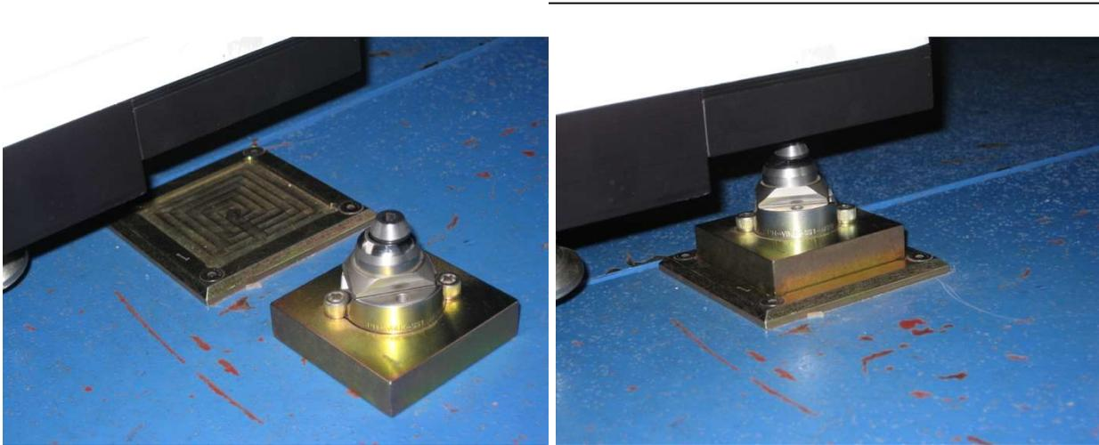
Figure 3: The spherolinder base plate and assembly are shown in the left photo. The assembly has been placed in the base plate in the right photo.
