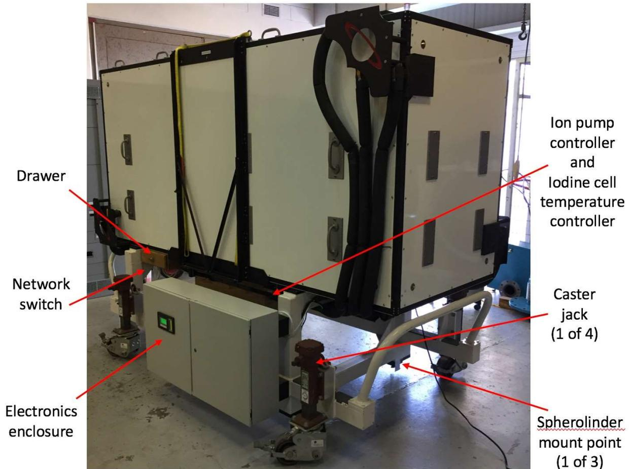
Figure 1: The side of PFS that faces the edge of the Nasmyth platform.
