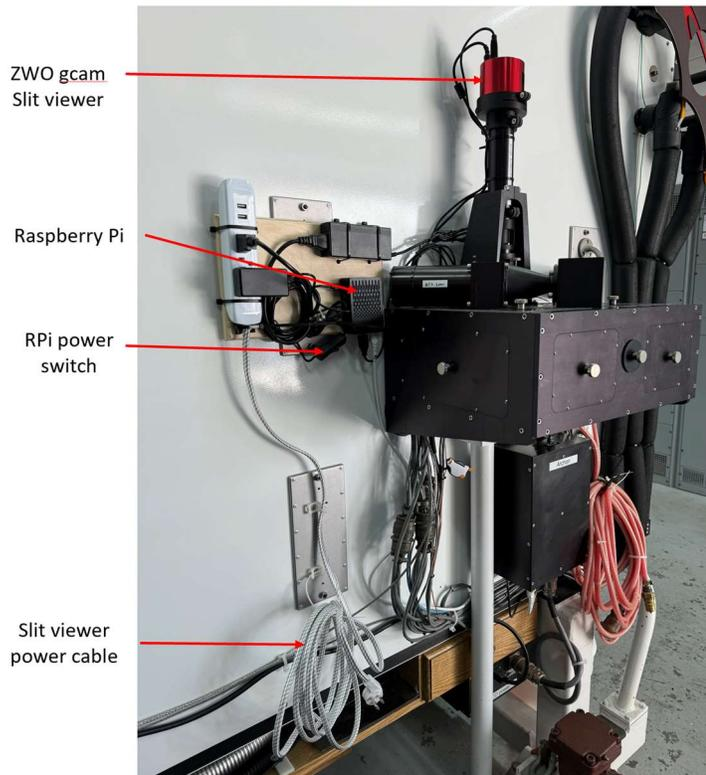
Figure 5: Slit viewer components.
